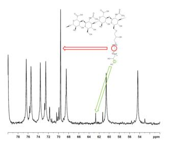
Figure 3: 13C spectrum of PEGDE crosslinked hydrogel after enzymatic digestion limited to the 50-80 ppm range (sample #1)
