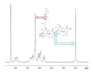
Figure 1: 1H NMR spectrum of PEGDE crosslinked hydrogel disaccharide unit after enzymatic digestion (sample #1). Signals due to the protons in the repetitive unit –C2H4O– in PEG (red) and to the methyl group on the HA chain (blue) are evidenced. The signals from the remaining 10 PEG protons overlap the HA ones (3.2-4.0 ppm) completely
